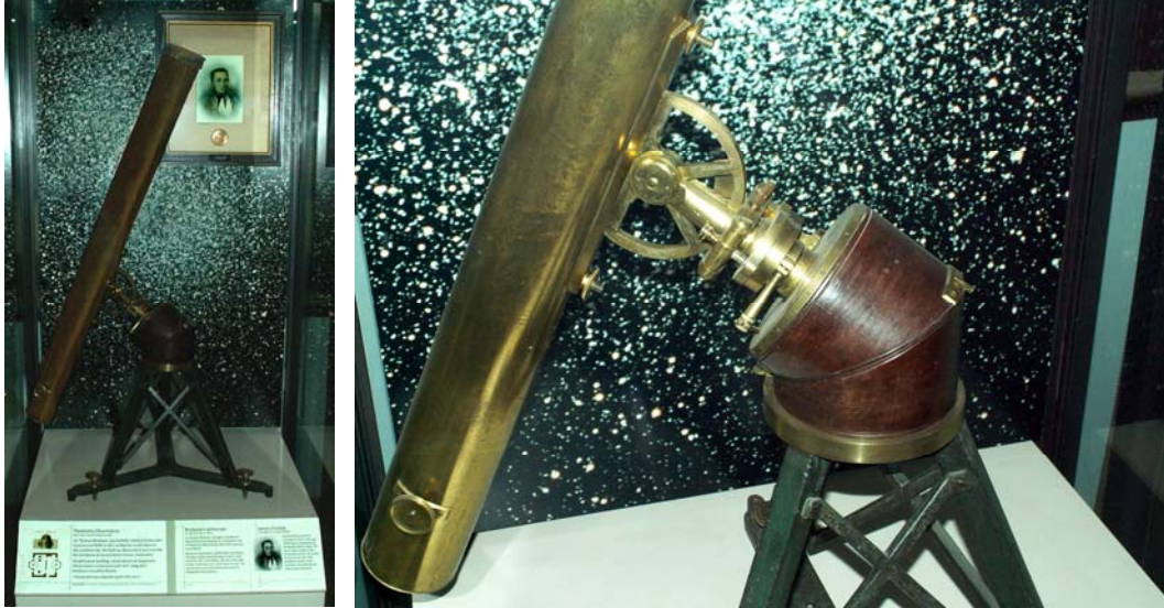
Plate 3.27: The 3.25-inch aperture, 46-inch focal length, Banks equatorial achromatic telescope, and mounting detail, now located at the Sydney Observatory. 244
