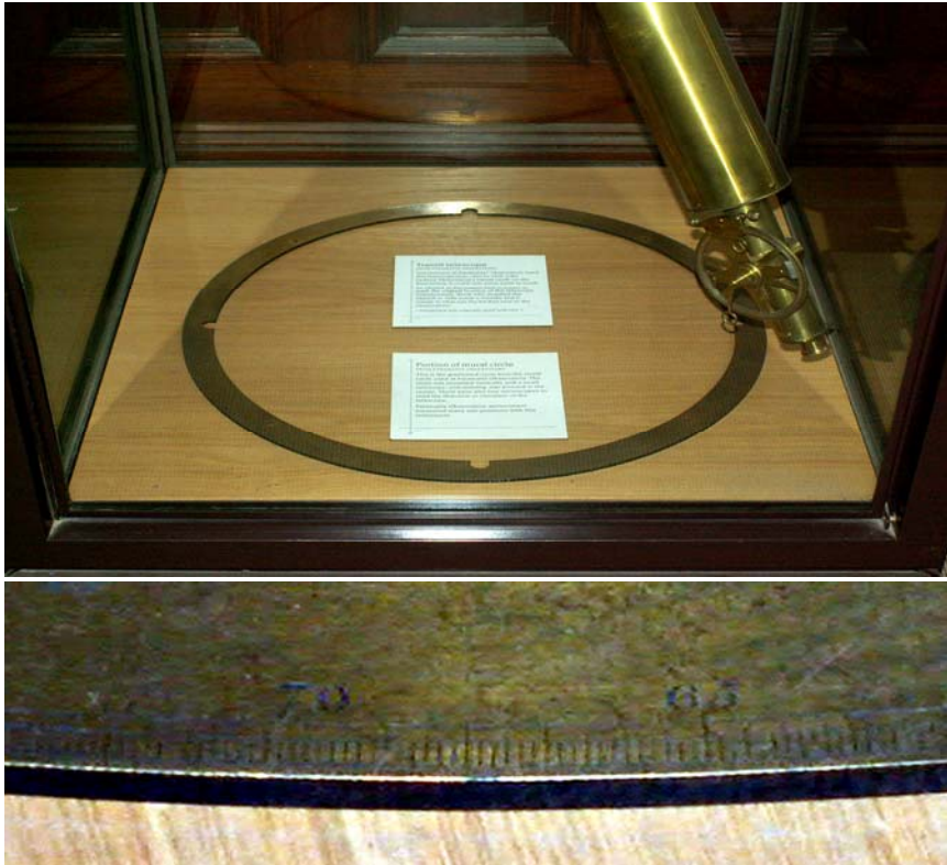
Plate 3.26: Part of the 2-foot diameter mural circle and an enlargement of the circle showing 1 degree = 6 divisions. 234
