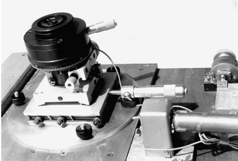
Fig. 21.6 The RETEL micrometer attached to the 205-mm reflector of Jean-François Courtot (J.-F. Courtot)
