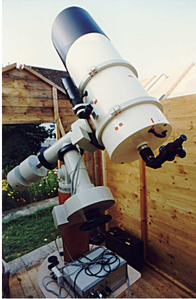
Fig. 21.7 Fig 20.8 The 32.5-cm Cassegrain of Andreas Alzner fitted with a Double Image micrometer. (A. Alzner)
