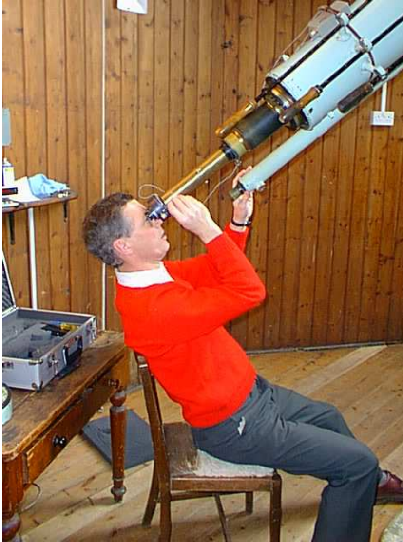
Fig. 13.1 Fig. 15.2 A RETEL micrometer fitted to the 8-inch refractor at Cambridge. The Barlow lens assembly is the brass tube immediately above and the power supply for the field illumination is attached to the tube within reach of the eyepiece. Comfortable observing positions such as this are rare. The chair collapsed entirely soon after this picture was taken!
