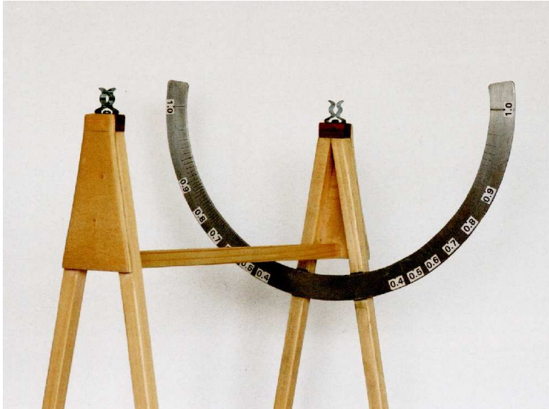
Fig. 14.4 Metal clamps serve as bearings for the grating frames and allow a quick exchange of frames. Note the cosine scale for reading the frame inclination.
