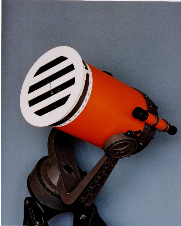
Fig. 14.1 The author's 20-cm Schmidt-Cassegrain equipped with a 50-mm grating. The first-order images are 2.3 arc seconds from the zero-order image. See also Fig. 14.5a. The position angles can be read on a 360 degree scale
