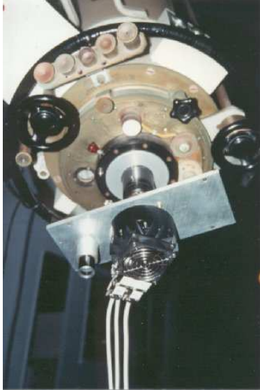
Fig. 21.3 The plate at the back of the refractor can be shifted in the focal plane. It supports both the CCD camera and the eyepiece used for visual control of the field (Courtesy R. Gili).
