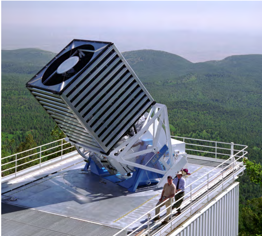
Fig. 12.1 Sloan Telescope New Mexico. The unusual shape of this telescope is due to its wind shields. When the telescope is not in use it is covered by a movable shed that runs on the tracks leading off the bottom left of the picture. Image credit: Fermilab
