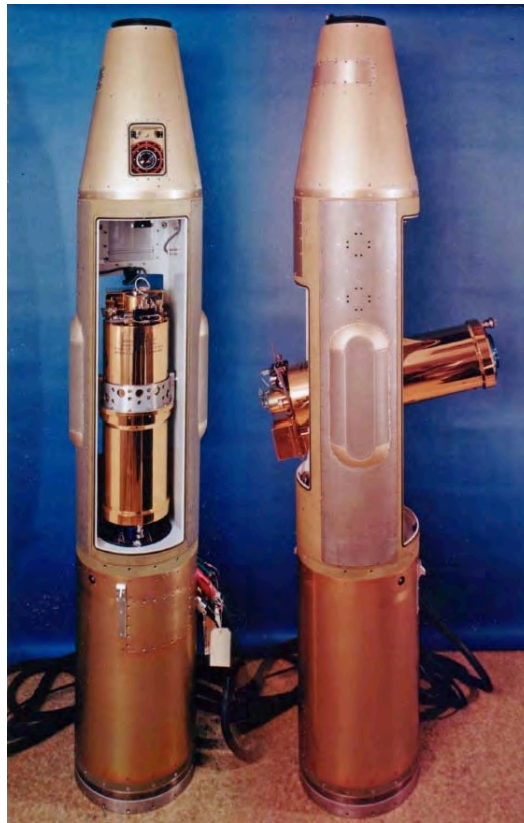
Fig. 6.5 AFGL Aerobee rocket payload showing the telescope in launch position ( left ) and in an observing position ( right ). The overall diameter of the rocket is 45 cm; the telescope mirror diameter is 16.5 cm. Image credit: Springer Publishing Company
