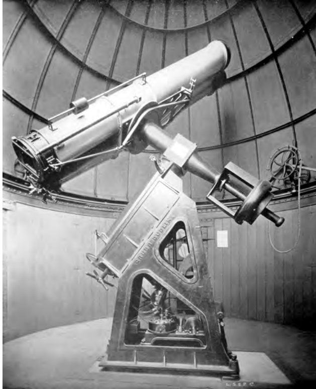
Fig. 4.3 One of the telescopes used to make the Carte du Ciel—the 13-inch astrograph at Greenwich Observatory, London in about 1900. Image credit: Graham Dolan
