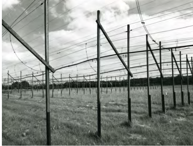
Fig. 5.9 Part of the 4-acre radio telescope at Lord's Bridge Observatory with which pulsars were discovered in 1967. Image credit: University of Cambridge
