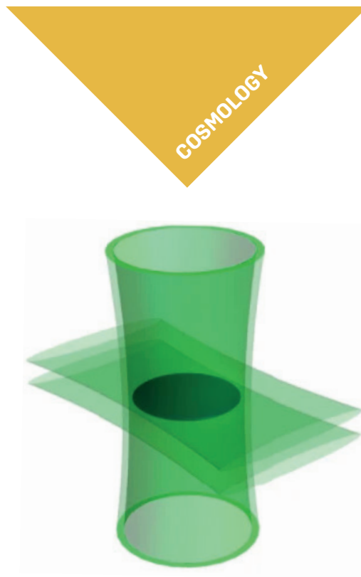
Fig 1. The planned experiment uses a “box trap” made of laser light to confine ultra-cold atoms into a 2D plane. Image from Navon N. et al., Nat. Phys. 17, 1334–1341 (2021).
