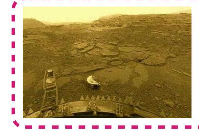
The Venera 13 lander had cameras to take pictures at the surface, a springloaded arm to measure how hard the surface is and a microphone to measure how fast the wind is.
